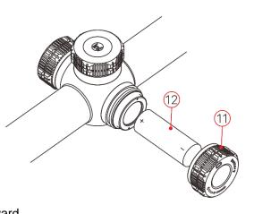
• Close the battery compartment cover (11) by turning it clockwise.
