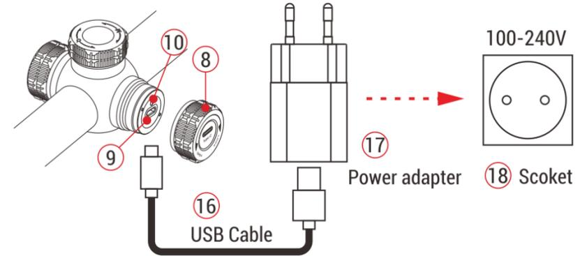
**Note:** The USB port can only be used for charging the built-in battery pack
