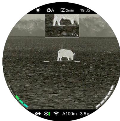
hold the **Image Mode button (6)** to turn on the PIP function.
