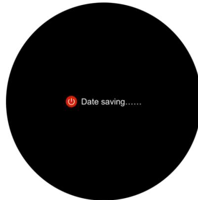
and the device is off. **When the device is powering off and saving data, do not disconnect it from its power source.**
