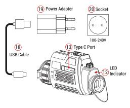
LED indicator displaying the current status of the device
