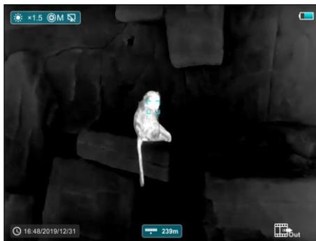
short press the **Up/Ranging (5) button** is required for ranging.
