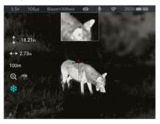
d. When the reticle matches the POI, long press the Menu button to save the reticle position.
