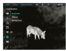
There are three calibration modes: Auto Calibration (A), Manual Calibration (M) and Background Calibration (B).
