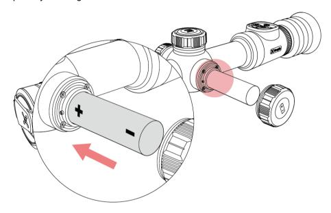
Note: The replaceable 18650 battery should be charged using a separate battery charger and cannot be charged via the BOLT's Type C interface.
