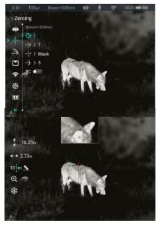
distance, and shoot accurately at the target ,If you are unsure of the distance to the target, you can press the LRF button, and the rangefinder's distance will automatically update to the zeroing distance.
